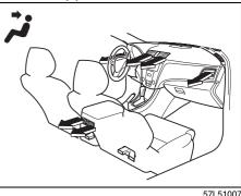
Temperature-controlled air comes out of the center, side and rear outlets.
